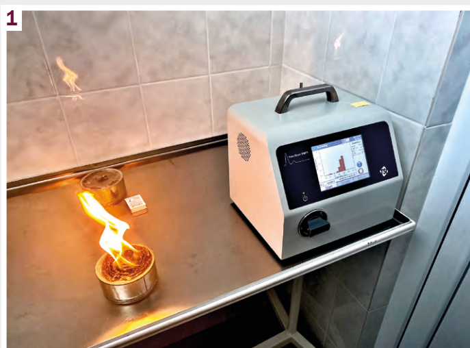
Fig. 1. Examination of ultrafine aerosol after the 10-minute trench candle burning using the portable scanning spectrometer NanoScan 3910 (USA).
